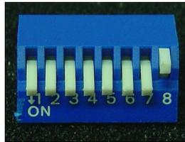
Channel sections 1-7 on, unused section 8 off.
