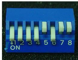
Channel sections 1-4 on, mode sections 5-7 off-on-off, unused section 8 off.
