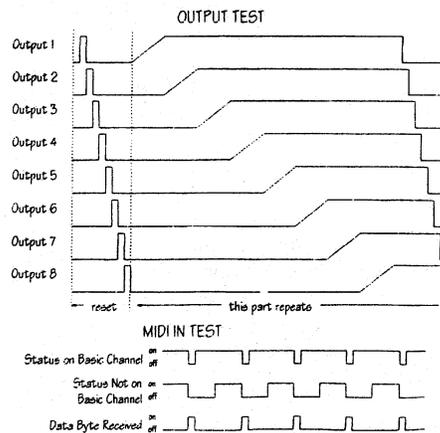
**MIDI In Test** - When MIDI data is received, the output test is interrupted and the MIDI In LED flashes brightly and regularly to indicate the kind of data that was received as shown at right. Reset to start the test again.
