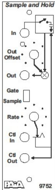
CV output, proportional to the sampled or gated input signal voltage. A random CV with noise as the input.
