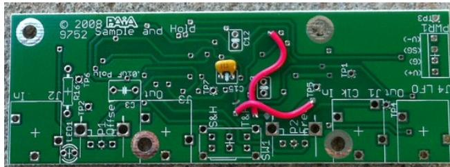
This first run of boards has some factory cuts/ rewires of connections from the Sample/Track switch to reflect the panel graphics.
