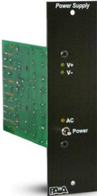
Build this dual-polarity, regulated 15 volt power supply for use as the power source in a fractional rackmount system of 9700 Series modules or other devices needing clean, stable, DC power.
