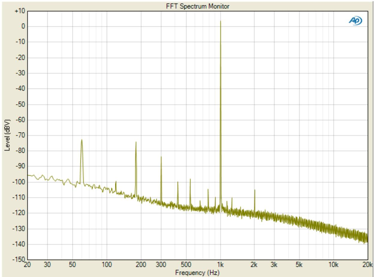
**Figure 1. FFT of 9802k for a 1kHz Input**
