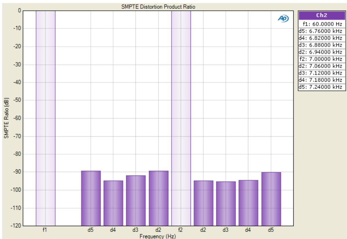
**Figure 9. SMPTE two-tone Intermodulation**
