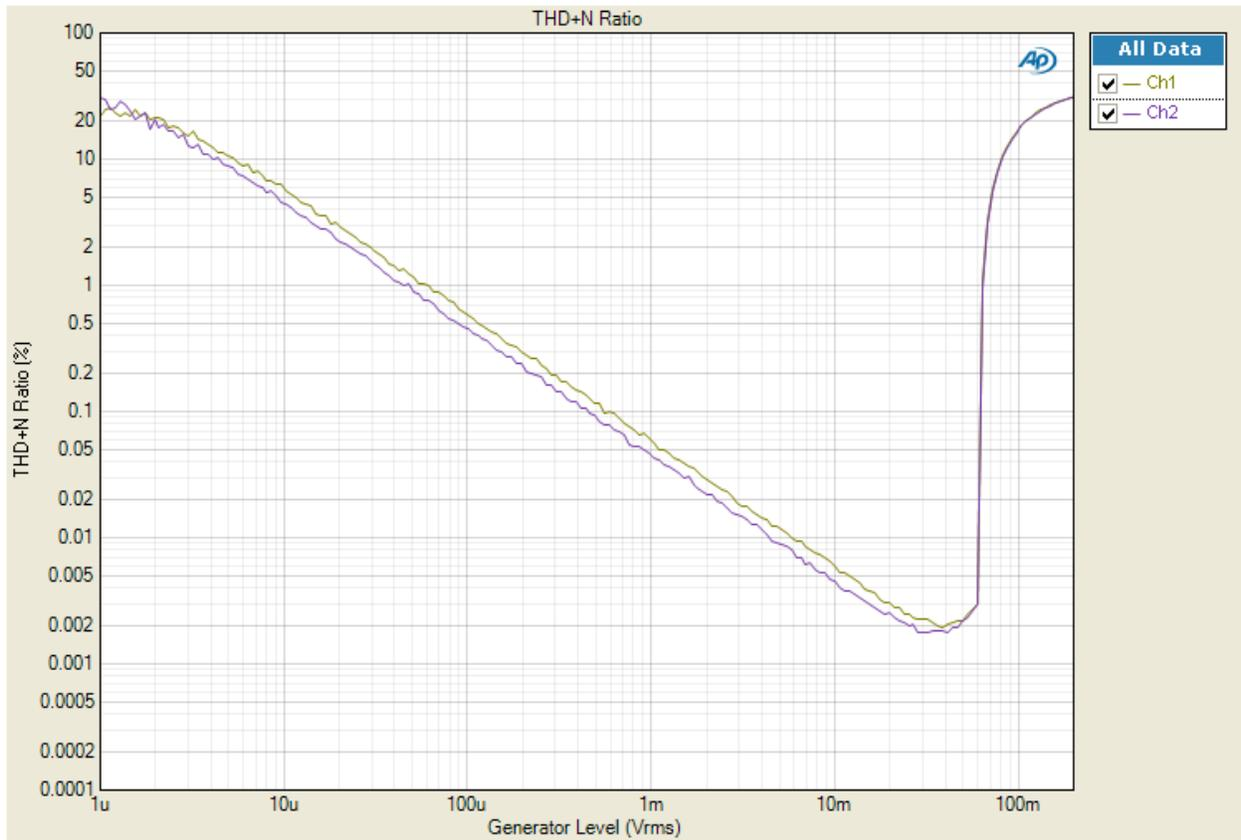
**Figure 4. Distortion vs input amplitude plot of 9802k**
