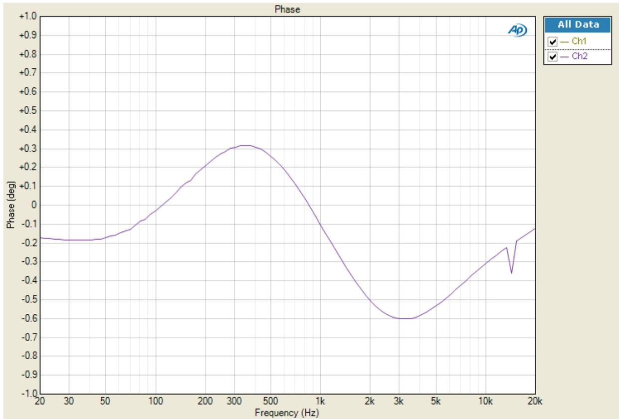
**Figure 8. 9802k Phase deviation vs. frequency**
