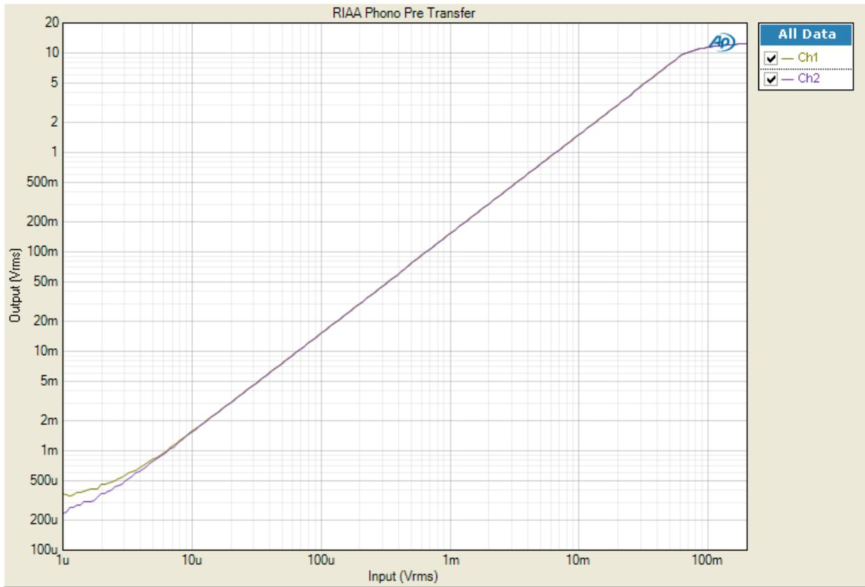
Figure 2. Voltage Transfer plot of 9802k
