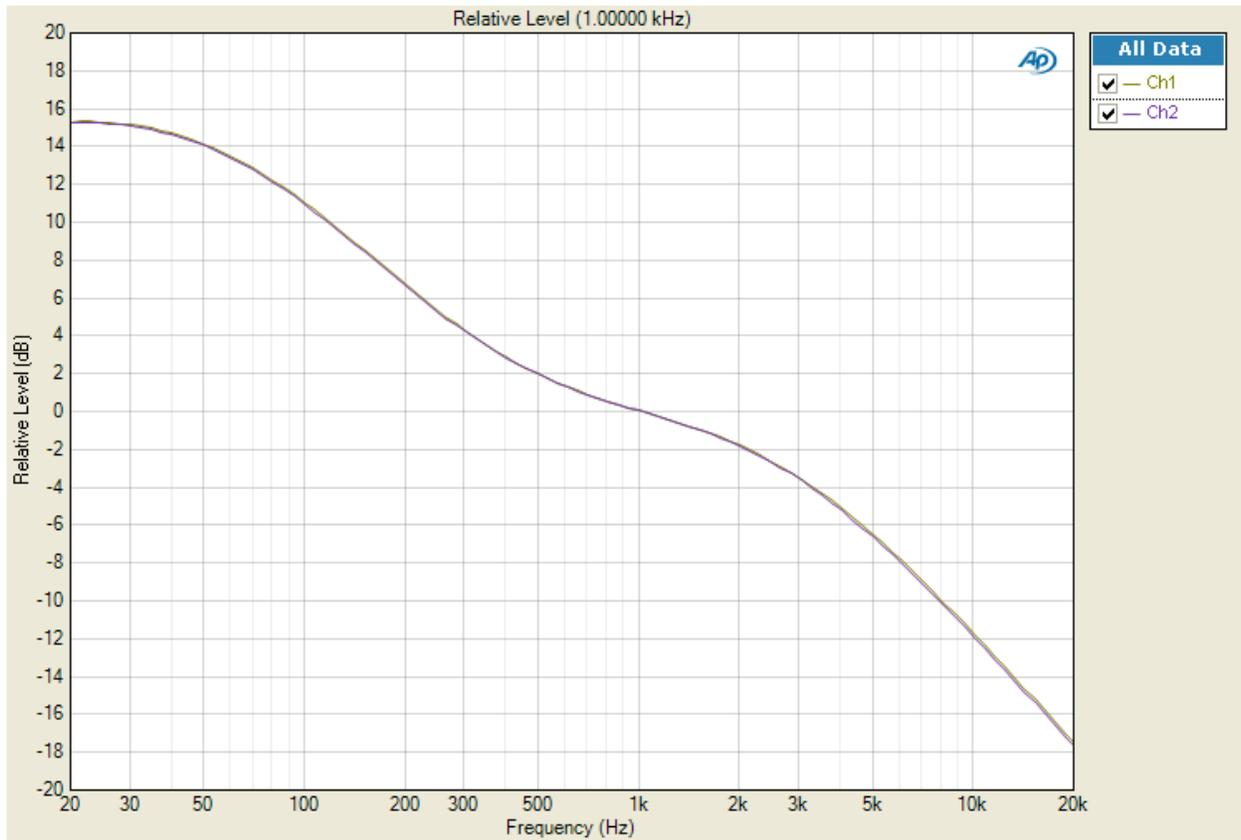
**Figure 6. 9802k frequency response, relative to 1kHz**
