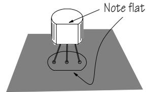
The straight line of the pc graphic symbol corresponds to the flat face of the transistor case.
