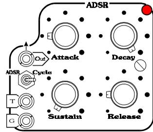
**Attack control.** This panel control sets the rate at which the ADSR function increases during the Attack phase. Clockwise rotation of the control slows the rate which is variable from 500uS to as long as 10 seconds.
