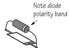
Diodes are also somewhat heat sensitive so the soldering operation should be done as quickly as possible.
