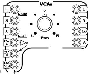
**PAN Control** - Sets the relative gain of the L and R VCAs. The linear control voltage response of the L and R VCAs means that for equal L and R inputs, Peak signal level at either the L+R or A outputs remains constant during panning.
