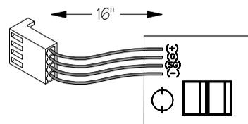
Use the 3 nylon wire ties to group the four wires together by placing one in the middle and the other two halfway to either end. Cinch the ties tight and clip off the excess.
