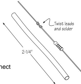
( ) Slip the length of sleeving from above over R115 and connect the free lead to J3-R. Bend back to secure. **Do not solder**.
