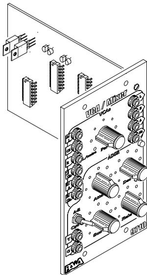
Ordinarily, Voltage Controlled Amplifiers are pretty routine. But by combining 2 VCAs, a Balanced Modulator, a White Noise Source and Envelope Generator in a single module and interconnecting them with a powerful normalization design, the 9710 redefines what a VCA module should be.
