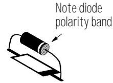
Diodes are also somewhat heat sensitive so the soldering operation should be done as quickly as possible.
