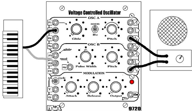
L and R inputs of a Stereo Amp switched to Mono can be used as shown in the illustration.
