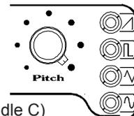
**OscA Pitch CV Input 1.** This 1V/oct scaled
