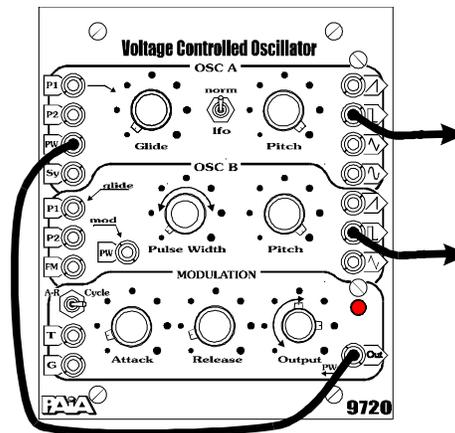
Set the Pulse Width control to the CCW limit and adjust the Modulator's Attack and Decay control so the output LED shows a cycle time of a second or so. While listening to OscB pulse output increase Modulator output level and observe PWM effect. Observe that rotation of the Modulator Output control CW beyond the 3 o'clock cause the output to be silent for a part of each Modulator cycle.
