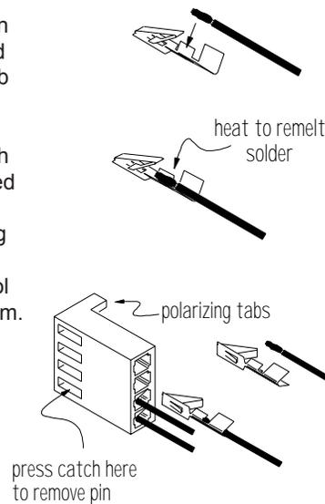
*If the wire comes loose, don't panic. The pins can be released from the connector by using a knife blade or small tool to reach through the slots in the connector body to press down the catch.*
