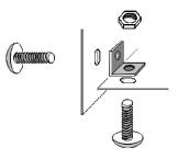
Use threaded hole of L-Bracket for mounting to FRBlank panel.
