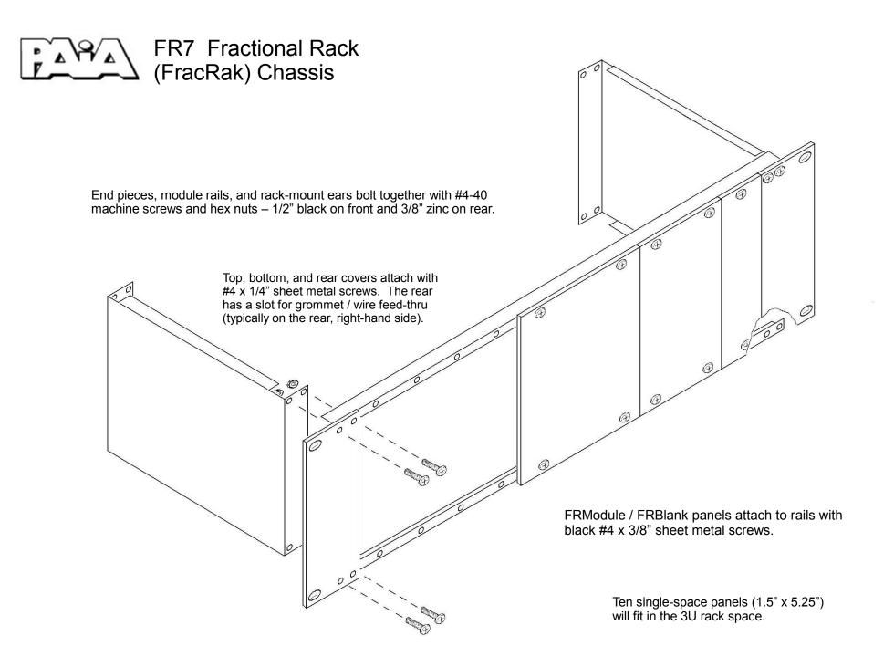
Note: The end pieces have additional holes which may be used for pots, jacks, or other purposes as desired. Be aware that power connectors can have one terminal common to the chassis and this can be a conflict when bringing in AC power where one wire is used as a neutral, circuit-common/ground. Remove any finish protecting film before assembly. For best alignment, hand-tighten nuts and bolts until all in place, then fully tighten.
