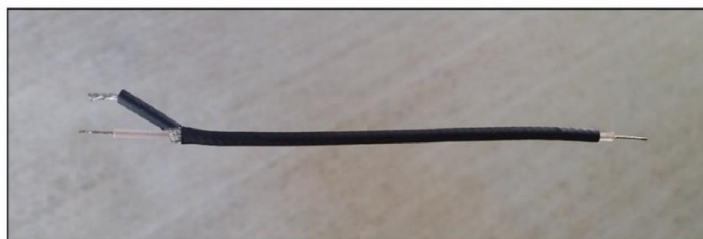
Prepared Shielded Cable (stripped insulation covers shield)
